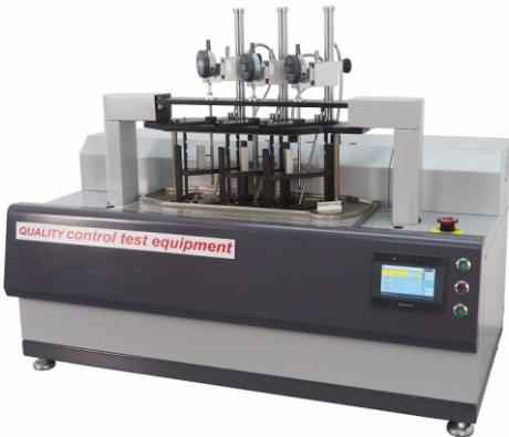
■ ZGT HV 3000 D3 is a lightweight and compact HDT/VICAT tester. It is designed to measure heat deflection temperature and VICAT softening temperature for evaluation of thermal property of plastic materials.
